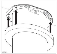
Finally, being careful not to scratch the chimney, push the cover plate up and onto its locking pins until it clicks into place. If installed correctly, the cover should be secure and flush against the ceiling.
